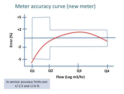
Q1 = minimum flowrate at +/- 5% Q2 = minimum flowrate at +/- 2% Q3 = permanent flowrate Q4 = maximum flowrate
