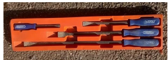
Advised tools for the removal of chamber covers
